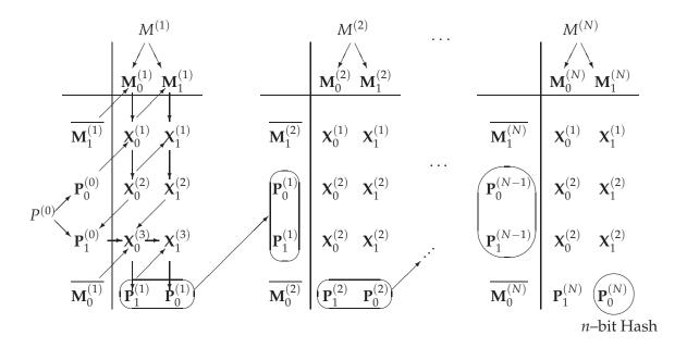
**Figure 2.1:** A graphic representation of the EDON- $\mathcal{R}$  hash algorithm.
